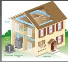
The diagram shows a cross-section of a two-story house. A furnace is located in the basement, connected to a network of ducts that run through the attic and into the rooms. An air conditioner is shown on the exterior wall, also connected to the duct system. A heat pump is shown in the basement, which can both heat and cool the house. Labels include 'Furnace', 'Air Conditioner', 'Heat Pump', 'Ductwork', 'Attic', 'Basement', and 'Rooms'.
