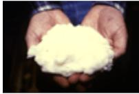
First, wood chips or recovered paper are combined with water and sometimes chemicals and "cooked" until the cellulose fibers separate from each other. This mushy solution of water and fiber is called pulp. This picture shows a handful of dry pulp. Sometimes, fillers and additives are added to the pulp to make the finished paper more glossy, absorbent, or water resistant.
