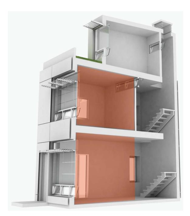
**INSULATING SHUTTER:** -during night, light shelf turns into insulating shutters, reducing heat
