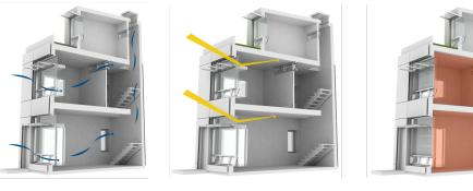
For our site we are using what is called the 'checkerboard' solar access plan. This staggers the placement of the structure on the lot. The first lot has the structure at the front setback line while the second lot has the structure at the rear setback line. This eliminates shadows from covering neighboring building facades.
