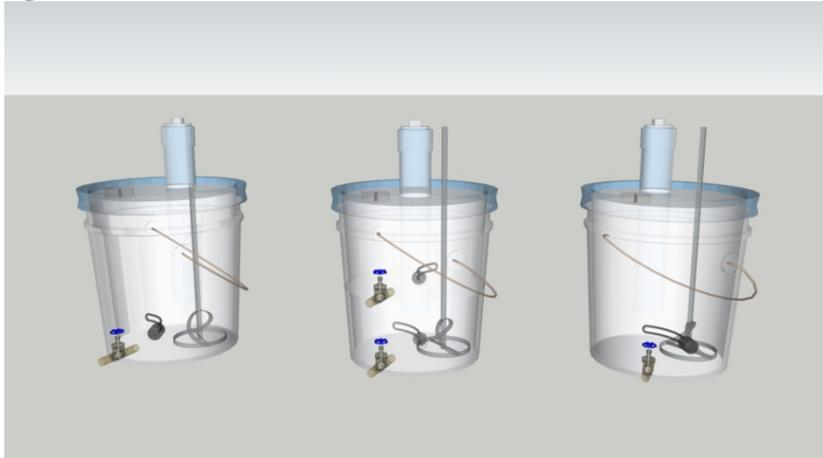
The picture above shows the three buckets, with feeding tube, heating elements, mixing stick, and drains installed.
