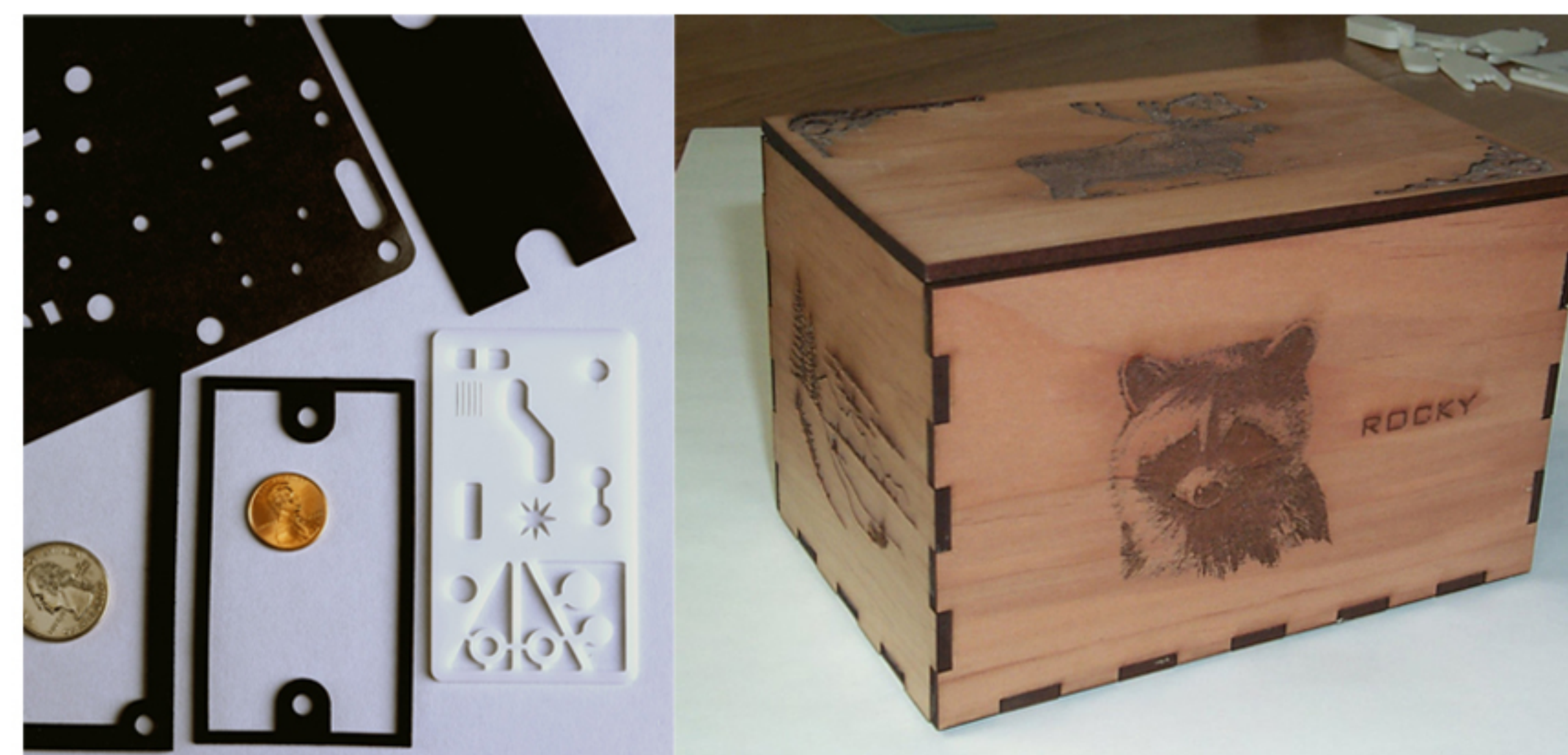
Figure 1: High speed laser machining of composite plastic, fiberboard, rubber, paper, etc. Figure 2: Wooden box precisely cut and decorated from one flat piece of wood using one simple graphics file.
