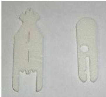
Laser cut foam components to verify design prior to expensive die procurement.
