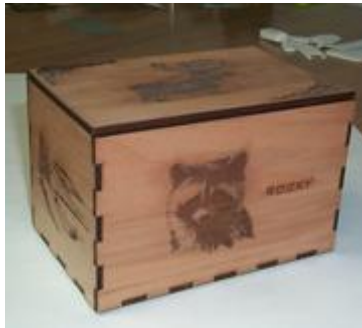
Wooden box precisely cut and decorated from one flat piece of wood using one simple graphics file.
