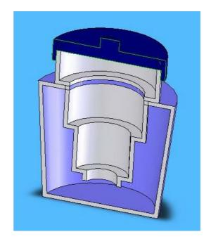
Figure 10.1.0.2. Cross-sectional view of container.
