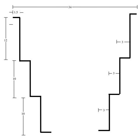
Figure 3. Dimensions of the filter housing, in cm.
