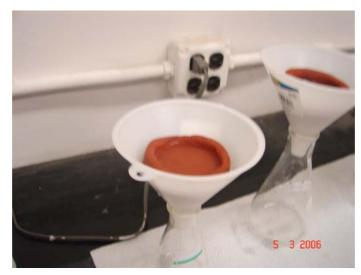
Figure 10. The setup of clay filters above flasks with the bacterial solution inside.
