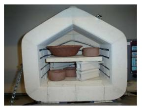
Figure 6. A picture of the kiln with some clay filters and a bowl ready to be fired.
