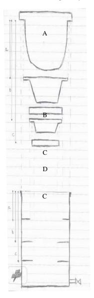
**Figure 10.1.2.3.** Filter structure for Design 2. A is the clay bowl filter; B represents the first plastic cone to direct filtered water away from the edges of the housing; both C's are clay filter disks; D is the second plastic cone.
