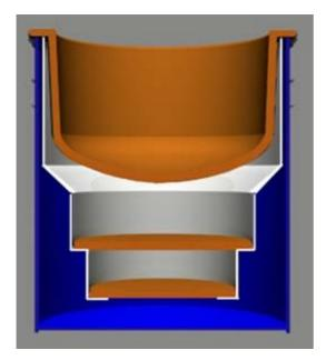
**Figure 1.** A colored side view of the filter housing in the bucket, with the clay pieces in brown.
