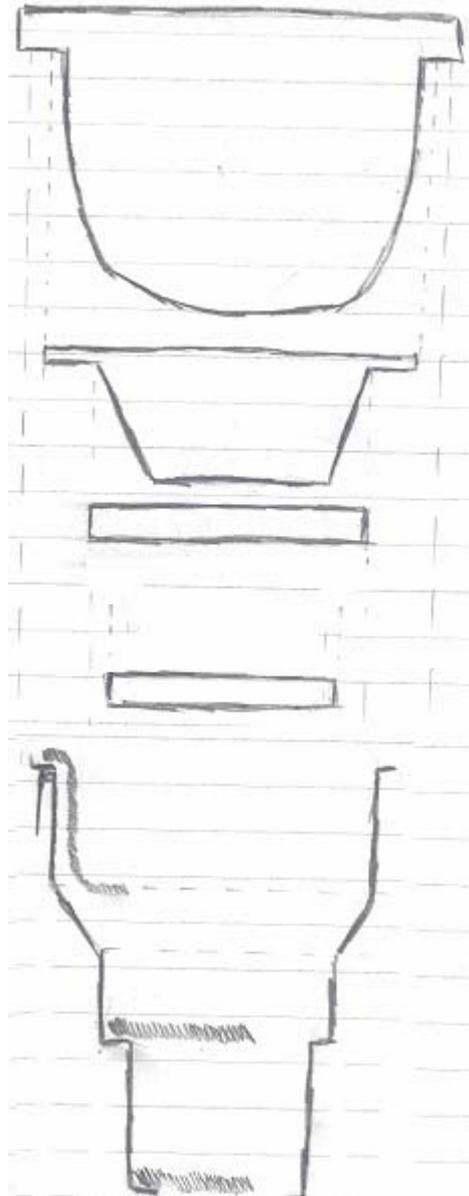
**Figure 10.1.6.1.** Last design. From top to bottom, the pieces are: clay bowl; plastic cone; clay disk 1; clay disk 2; plastic housing (shown with silhouettes of where the clay pieces will fit).
