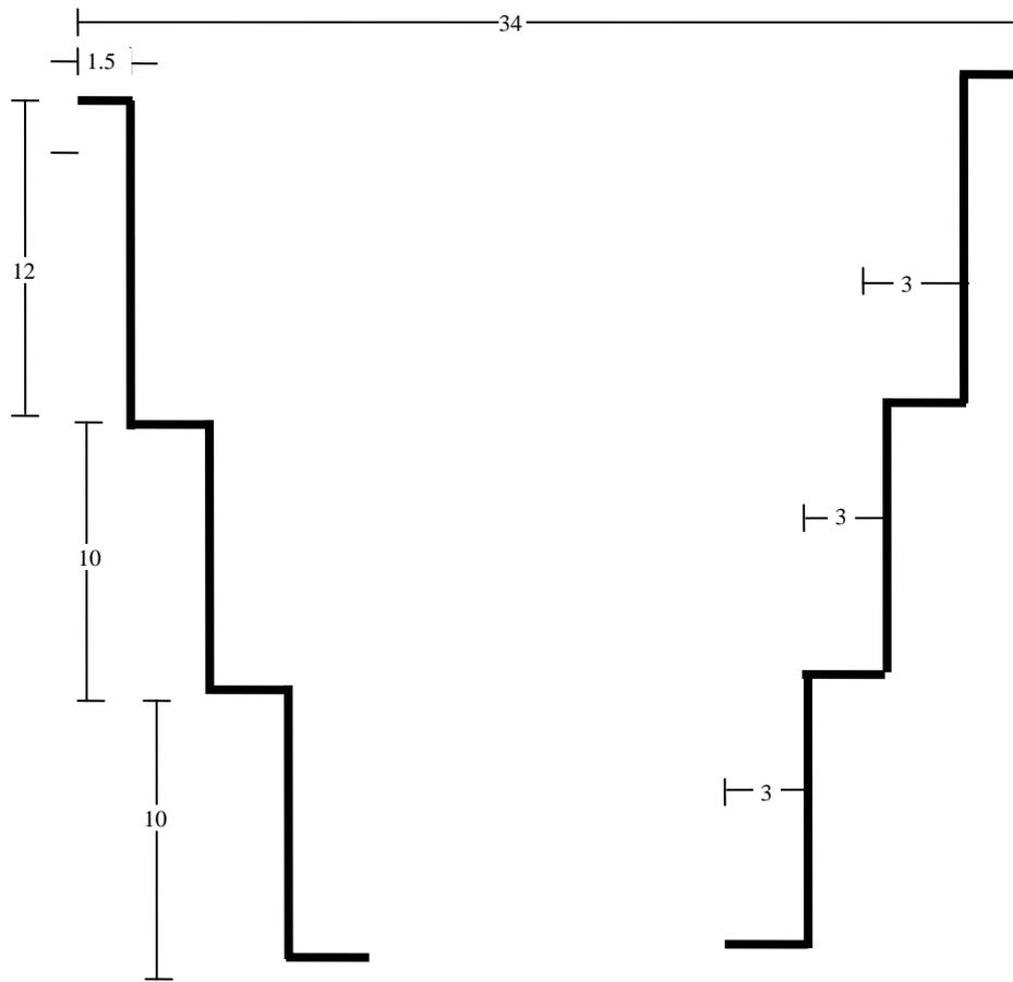
**Figure 3.** Dimensions of the filter housing, in cm.
