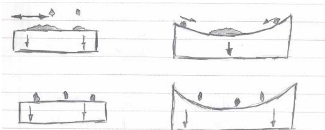
**Figure 10.1.2.1.** Suggestions for concave surface of disk. The disks on the right force water through the center if flow rate is slow enough.
