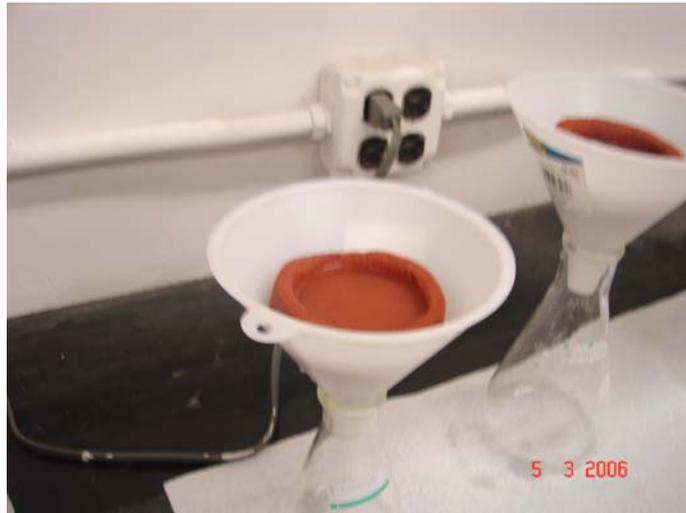
**Figure 10.** The setup of clay filters above flasks with the bacterial solution inside.
