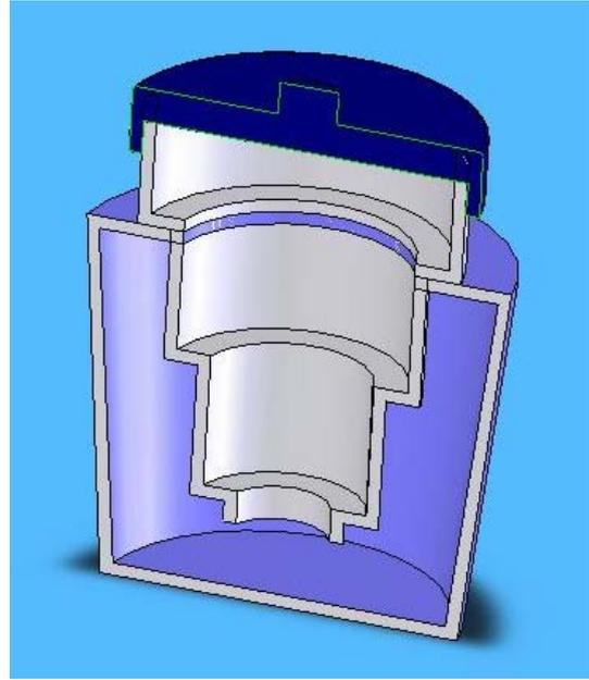
Figure 10.1.0.2. Cross-sectional view of container.
