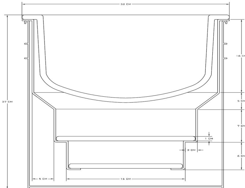
**Figure 10.1.3.1.** Dimensions and placement of disks in Design 3.
