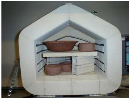
**Figure 6.** A picture of the kiln with some clay filters and a bowl ready to be fired.
