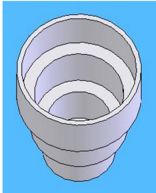
Figure 10.1.0.4. Filter housing.
