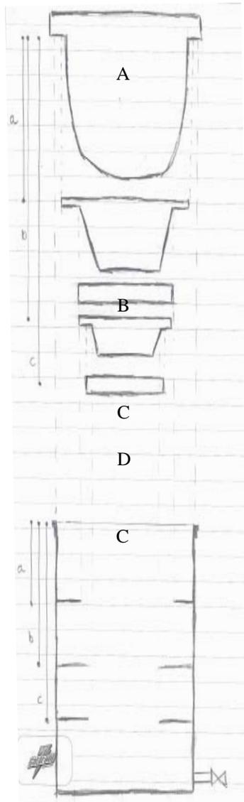
**Figure 10.1.2.3.** Filter structure for Design 2. A is the clay bowl filter; B represents the first plastic cone to direct filtered water away from the edges of the housing; both C's are clay filter disks; D is the second plastic cone.
