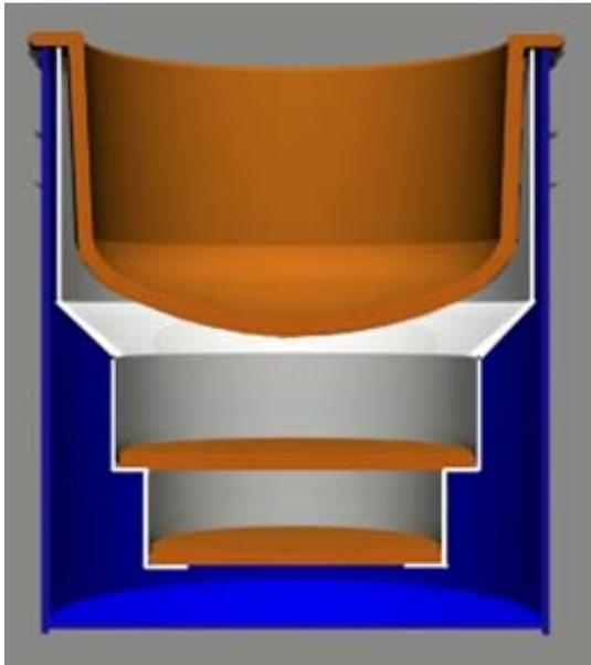
**Figure 10.1.3.2.** Cross-section of filter. Brown = clay.
