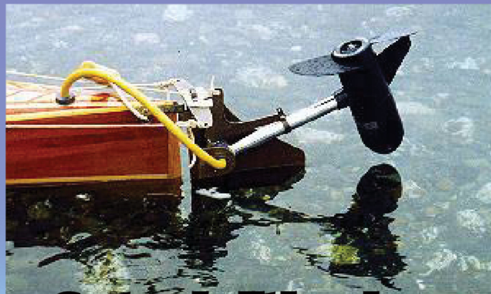
Custom built kayak and motor mount
