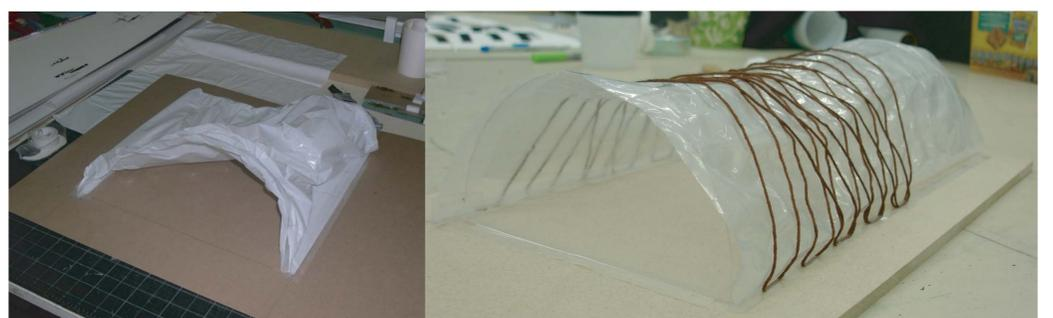
To give added rigidity and resistance to horizontal winds a cable net structure would be implemented. This structure would act as a tether to the ground keeping the greenhouse in place.
