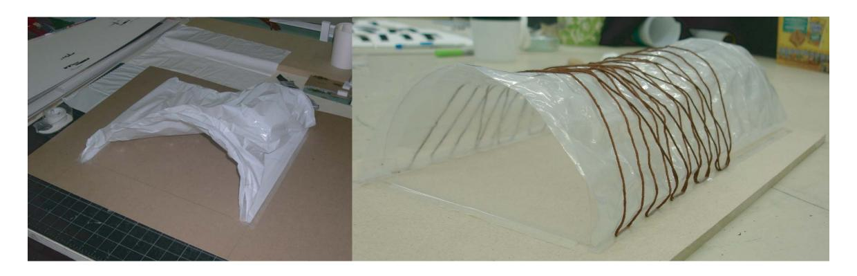
To give added rigidity and resistance to horizontal winds a cable net structure would be implemented. This structure would act as a tether to the ground keeping the greenhouse in place.
