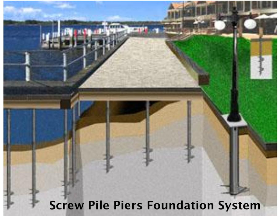
**Screw Pile Piers Foundation System**
