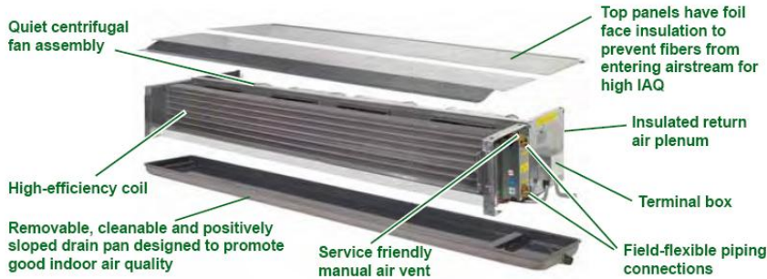
Picture of a ceiling concealed fan coil 3
