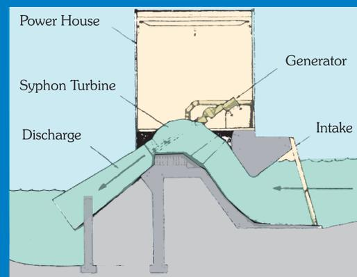
The S-Type Turbine, a cheaper alternative to traditional hydroelectric turbines.
