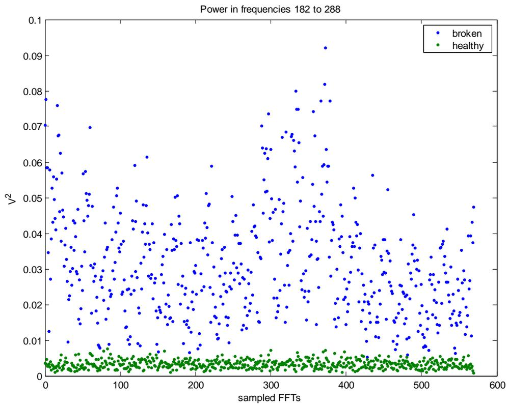
Figure 9: Amplitude of Broken and Healthy Data
