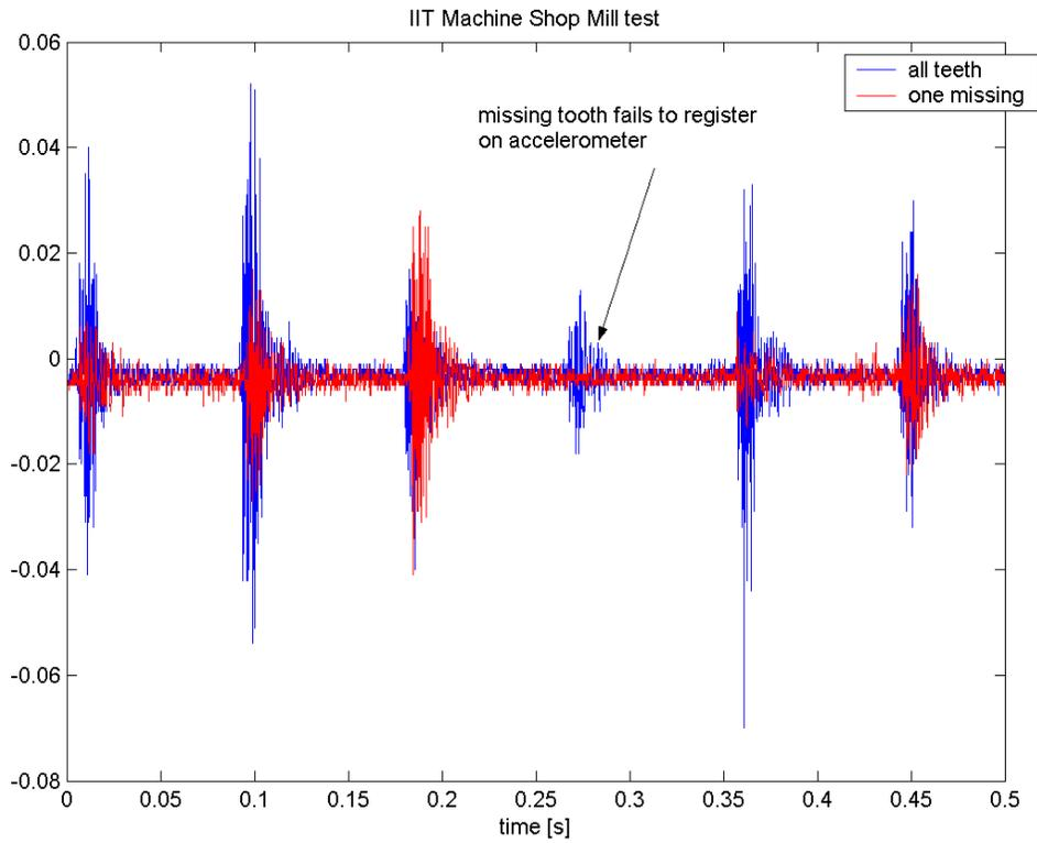
Figure 2: Data from the Mill at IIT taken at 10 kHz
