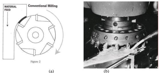
Figure 1: (a) Diagram and (b) picture of a mill
