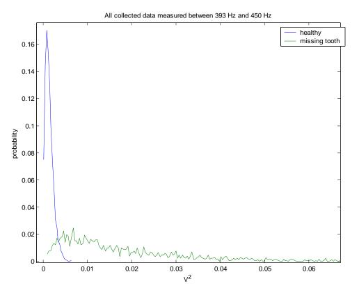
Figure 10: Probability of a Broken Tooth
