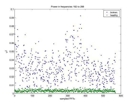
Figure 9: Amplitude of Broken and Healthy Data
