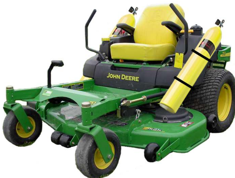
Figure 5. Hydrogen Tank Mounting System
