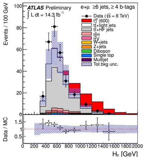
Fig. 3. Comparison between data and simulation for  $H_T$  in the combined  $e$ +jets and  $\mu$ +jets channels with  $\geq 6$  jets and  $\geq 4$  b tags. Also shown is the expected  $t't'$  signal corresponding to  $m_{t'}=600$  GeV in the  $t'$  doublet scenario. The shaded area represents the total post-fit background uncertainty [7].
