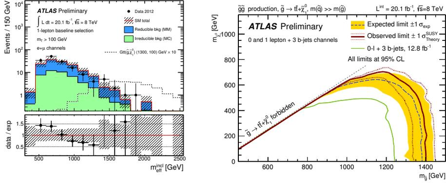
Fig. 5. (Left) The distribution of the inclusive effective mass for the baseline selection in the 1-lepton channel and after requiring  $m_T > 100$  GeV, as observed in data together with the background prediction from the matrix method. The prediction for one signal point from the  $Gtt$  model is overlaid. (Right) Expected and observed exclusion limits in the  $(m_{\tilde{g}}, m_{\tilde{\chi}_1^0})$  plane for the  $Gtt$  model [10].
