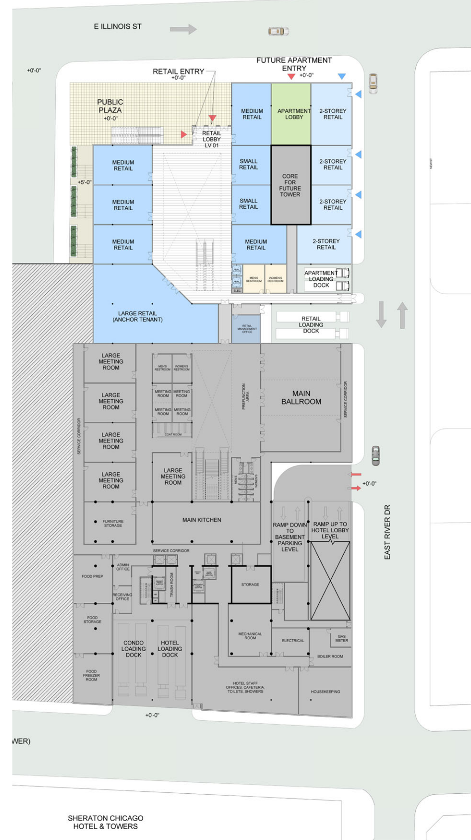
LEVEL 1 (+0'-0") Retail Podium Entry from Illinois St Hotel Ballroom and Conference Centers Back-Of-The-House Services, Loading Dock
