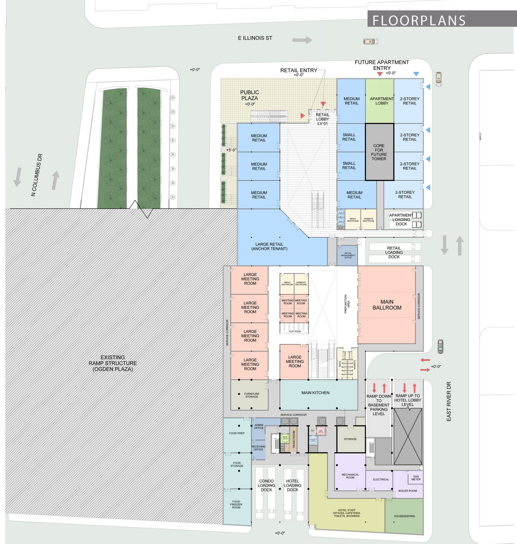
LEVEL 1 (+0'-0'') Retail Podium Entry from Illinois St Hotel Ballroom and Conference Centers Back-Of-The-House Services, Loading Docks
