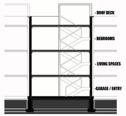
HOMES ARE STANDARD CONSTRUCTION WITH MASONRY COMMON WALLS FOR FIRE PROOFING. THE TYPES OF SPACES ARE BROKEN UP VERTICALLY WITH THE GARAGE AND ENTRY ON THE GROUND LEVEL, LIVING SPACES ON THE SECOND FLOOR, BEDROOMS ON THE THIRD FLOOR AND A ROOF DECK FOR AND OUTDOOR ENTERTAINING SPACE.
