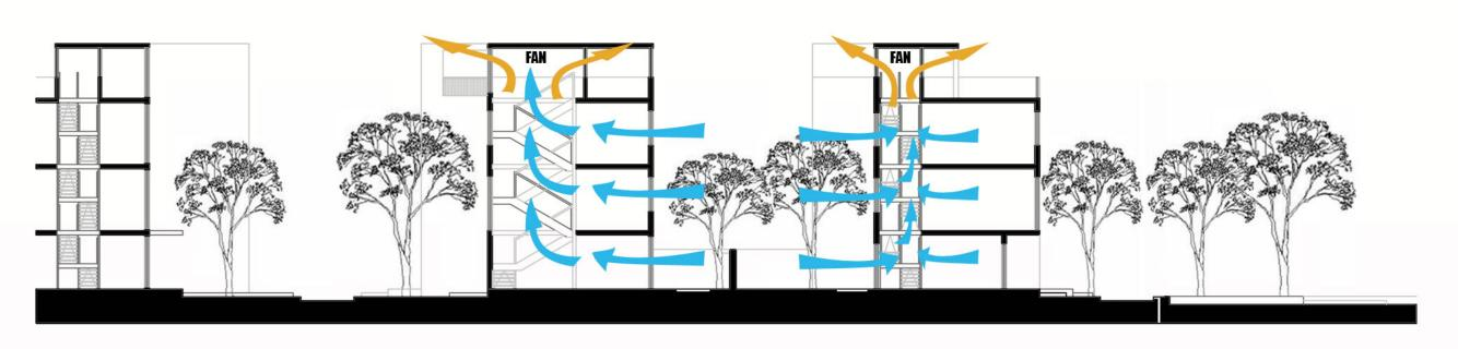
ABOVE: SECTION OF A TYPICAL BLOCK IN THE CLOSED CITY DESIGN
